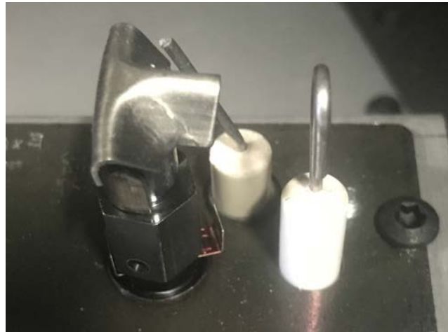
Figure 32: Correct Pilot Position
