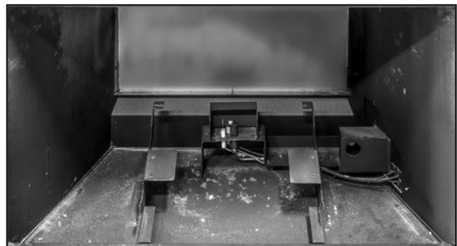
Figure 48: The rear liner can now be removed. Use a vacuum to clean up the bare firebox if needed.
