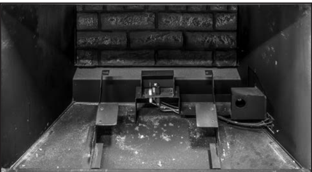
Figure 47: Lift the burner off the mounts and pull it out of the inlet box. The unscrew the panel brackets (T20's) from each side of the baffle to remove the left and right side liners.
