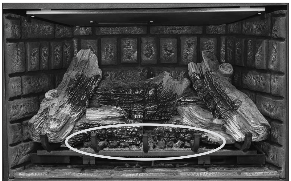
Figure 54: Pull apart Embaglow and spread a thin even layer over the burner area. Brush the ember wool as fine as possible (clump the wool together and separate it using the supplied brush) over the burner tube. Place coals on the air deflector in front of both mid logs as shown. Do Not cover the gaps between the burner and air deflector.
