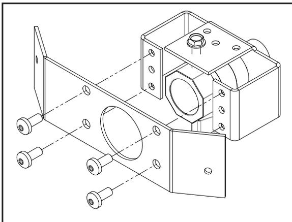
Figure 81: Gas Plate Removal
