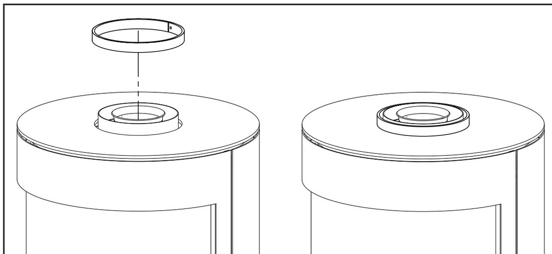
Figure 60: Top Plate Collar Placement
