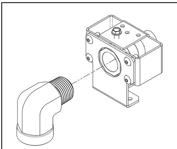
Figure 83: 1/2" Elbow Fitting Connection
