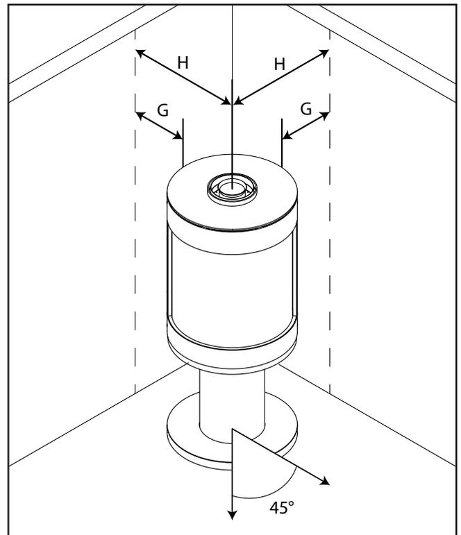
Figure 44: Clearance to Combustibles - Corner Install
