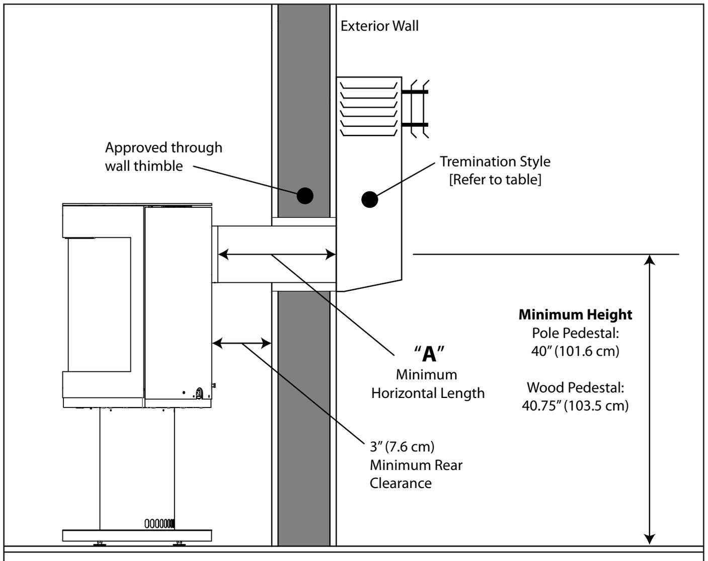
Figure 51: Minimum Vent Configuration - Rear Vent
