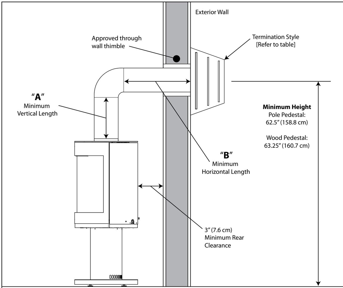
Figure 48: Minimum Vent Configuration - Top Vent
