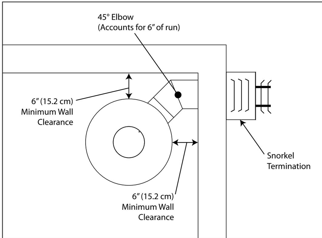
**Figure 52: Rear Vent Corner Install Venting - Top View**
