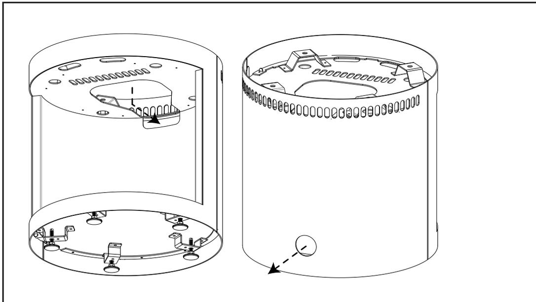
Figure 86: Wood Pedestal Gas & Electrical Rerouting
